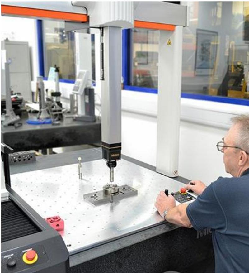
The rising volume of components being produced in A&M's machining facility recently began to place a strain on the business' Coordinated Measuring Machine (CMM) provision.
